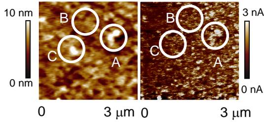
Fig. 1. The topography (left) and current (right) images of the MEH-PPV film. The tip bias is +4V.
