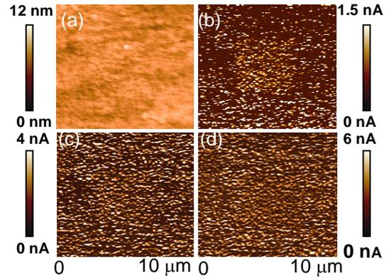
Fig. 5. With +2.5 V repeat scanning on the  $10 \times 10 \mu\text{m}^2$  area. The topography image (a) and the current images of first time scanning (b) the second time scanning (c) the third time scanning (d).
