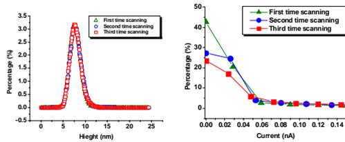
Fig. 4. Topography (left) and current (right) statistics of repeating bias with +2.5 V on  $5 \times 5 \mu\text{m}^2$  area.
