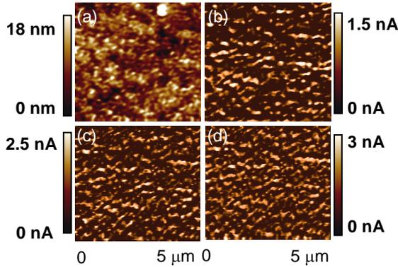
Fig. 3. With +2.5 V repeat scanning on the  $5 \times 5 \mu\text{m}^2$  area. The topography image (a) and the current images of first time scanning (b) the second time scanning (c) the third time scanning (d).
