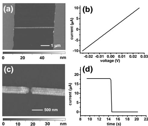
Fig. 4. (a) AFM image of a copper nanowire with a width of 120 nm, and (b) the corresponding  $I$ - $V$  curve that shows a resistance of 2.54  $k\Omega$ . (c) A pair of nanoelectrodes created by direct cutting a nanowire, and (d) the simultaneous obtained current versus time relationship.
