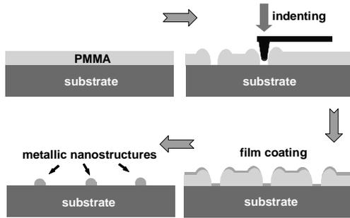
Fig. 1. Schematic diagram of the experimental procedure.
