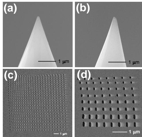
Fig. 3. SEM images of (a) a new tip, (b) the same tip after 625 indentations, (c) the resultant  $25 \times 25$  gold nanodot array, and (d) a gold nanodot array created by 4 different forces of 4.3, 5.6, 6.8, and 8.1  $\mu\text{N}$  (top to bottom for every 2 rows).
